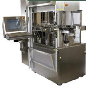
Huxley Bertram Servo-Hydraulic Compaction Simulator
