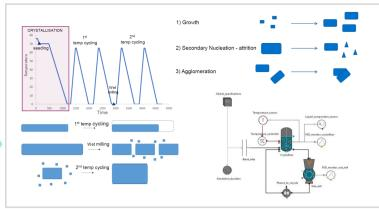
A finished 2D morphological population mass balance model implemented in gPROMS FormulatedProducts using crystallisation kinetic data may be able to predict quantitatively critical API characteristics such as particle size and shape, to better estimate flow properties around which crystallisation can be optimised.
