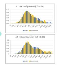
Many rate processes occur simultaneously during granulation. A population balance model implemented in PSE's gPROMS FormulatedProducts platform has been used to model the changing properties of the granules as the net result of these mechanisms. The model uses a combination of feed material properties (densities, size), equipment set-up (screw configuration and elements), and process settings (solid and liquid feed rates) as inputs and predicts the output granule particle size distribution.
